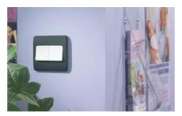
The Disabled Living Foundation recommends white switches on a dark background as being easier to distinguish for people with visual impairments. In some instances, it may be deemed necessary for the switch to contrast with the front plate, which in turn will need to contrast with the wall.
