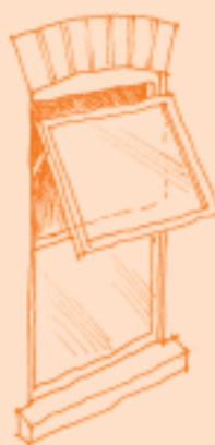
Replacement window in upvc: is fitted virtually flush with wall & has an opening system alien to the original. It also omits glazing bar
