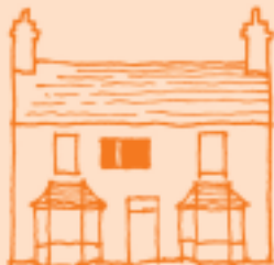
(b) The size & proportions of the new window ignores the symmetry of the elevation
